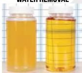
Contaminated ISO32 Turbine Oil: 1800ppm water ISO 20/19/17 Filtered Turbine Oil: 148pm water ISO ISO 15/13/10
